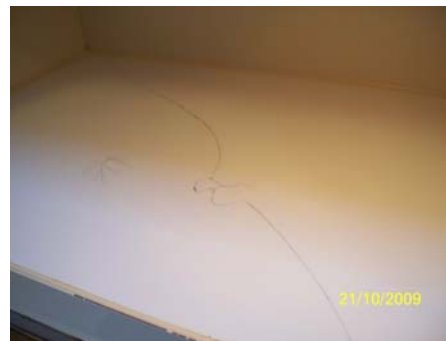
24.) Crack shelf in microwave.
